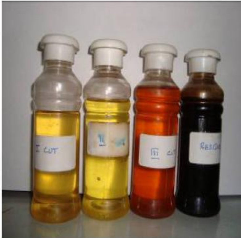
Different Fraction derived after Distillation of Our Crude Oil
