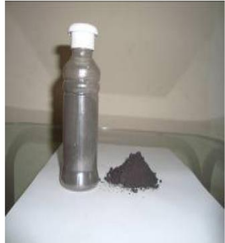
Solid Residue generated from PE Equipment
